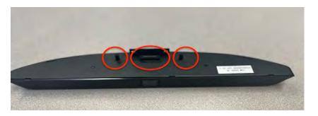
3. Secure the camera by attaching 2x Philips Head Screws included in the camera accessories box. These screws are attached on the back of the Whiteboard.
